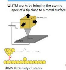
Through Current (I) – Voltage curves we find fingerprints about atomic and molecular spins
